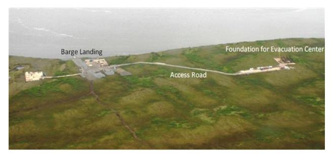
Figure 1. The beginning of a new village--Mertarvik Barge landing, Access road and evacuation center foundation (right). Photo: Harvey Smith, DOT/PF
