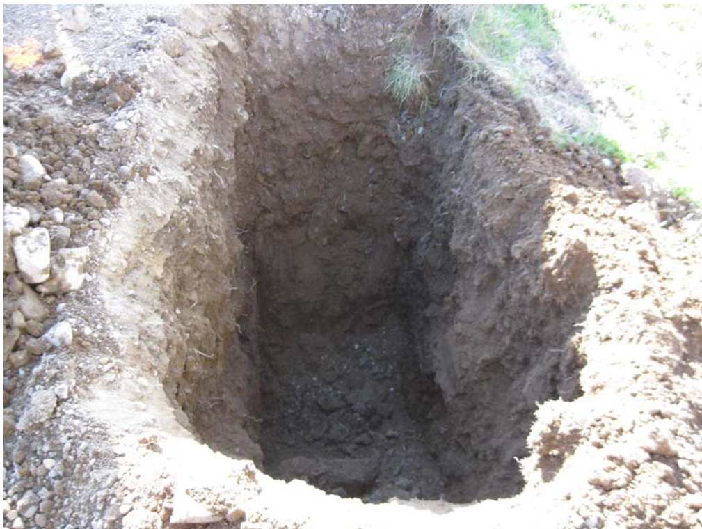
Photo 18 - TP-5 Soil Profile 5' BGS
