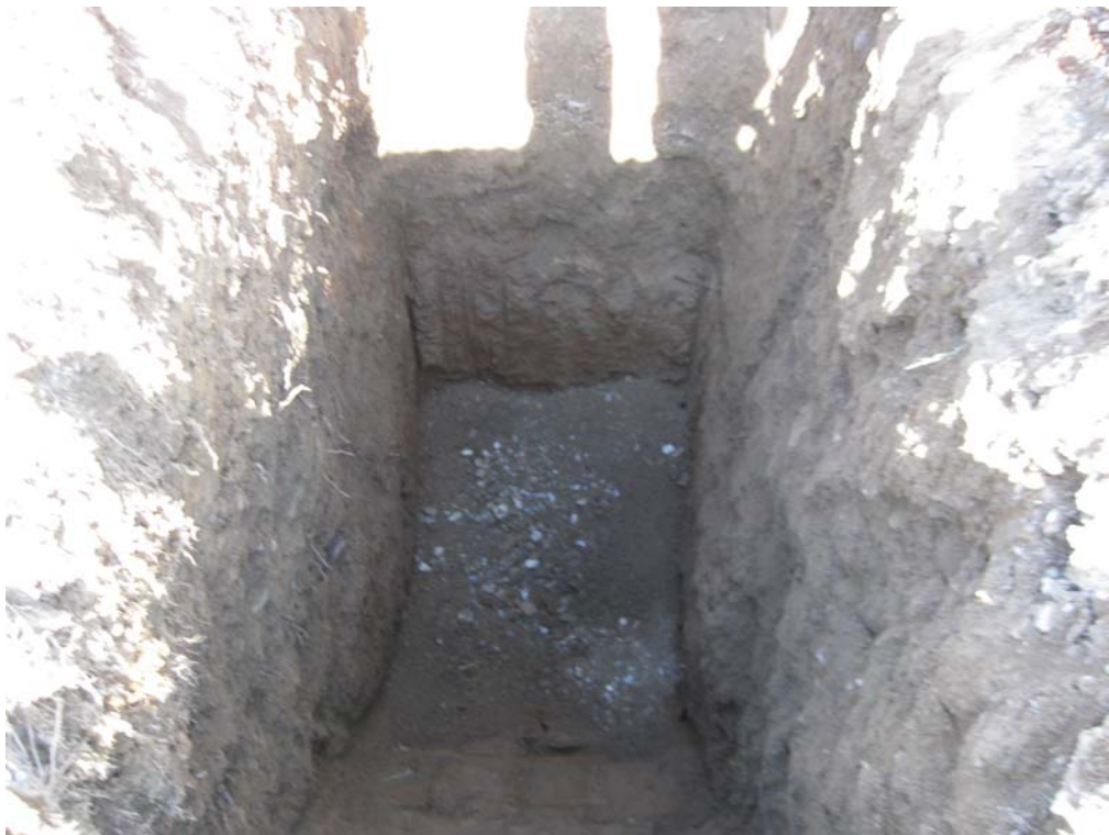
Photo 24 - TP-7 Soil Profile 6' BGS
