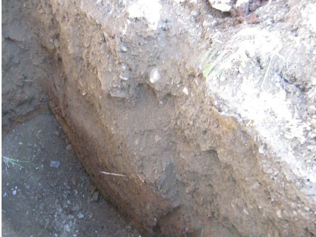
Photo 11 - TP-3 Soil Profile 5' BGS
