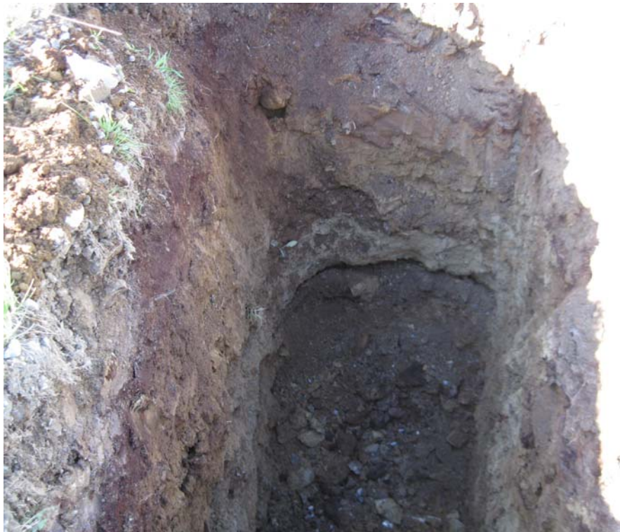
Photo 14 - TP-4 Soil Profile 5' BGS
