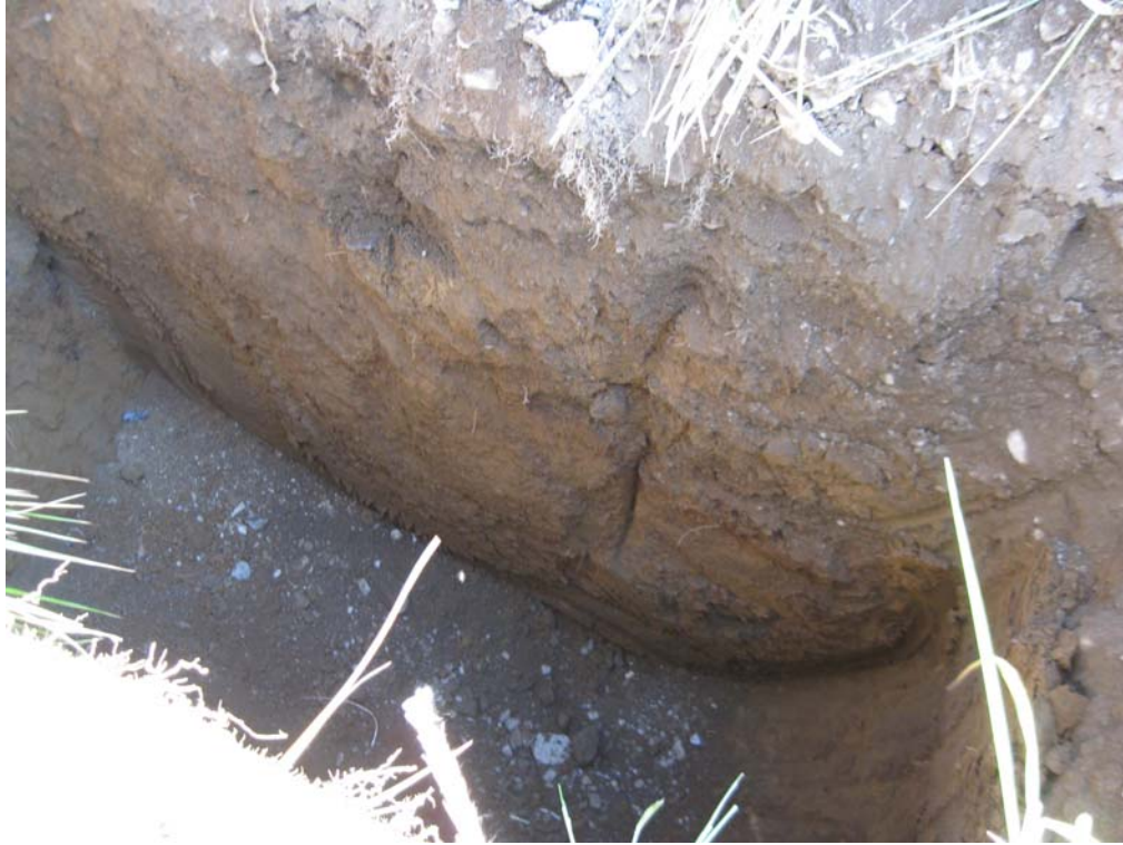
Photo 7 - TP-2 Soil Profile 5' BGS
